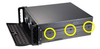
1. In order to install the rail, you must first remove the cover on the side. Three screws locate on each side.
